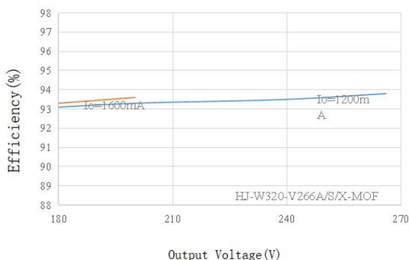
Fig. 14. Efficiency VS Output Voltage (Vin=120Vac)
